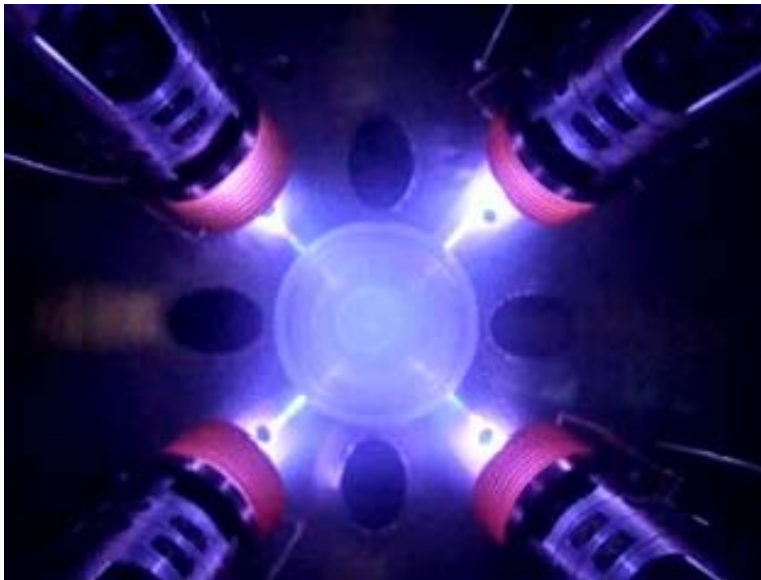
Figure 9: Photograph showing the plasma glow during the firing of the MEEVA arc plasma injectors.
